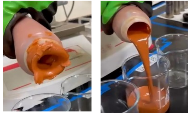
Figure 4. Pictures of flowability tests at 700 g/L. Left: type d, Right: type A.
